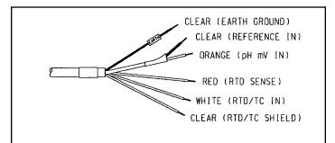
FIGURE 2-8. Models 396, 397, and 398 Option -62 for Wiring to Models 1054, 1181, 2081, 54, 81, 3081, 4081, SoluComp, and 2700 Preamplifier (PN 23054-03). Also for use with remote Junction Box PN 23555-00.
